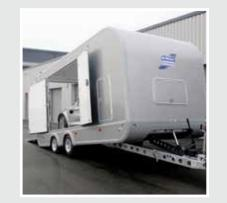
1. **Tilting Drawbar** To aid loading vehicles with low ground clearance.
