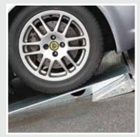
**3. Ramp Skid Extenders** Pair of ramp skid extenders to aid loading of vehicles with low clearance.
