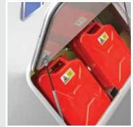
Front Wall Access Hatch The front wall access hatch allows for easy access to the front storage cabinet.
