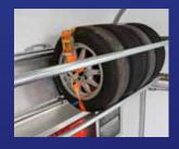
**Tyre Rack** Mounted to the front of the trailer this adjustable rack can accommodate a set of differently sized wheels/tyres.
